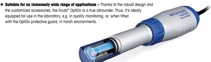
■ **Blochemical oxygen demand (BOD)** — The BOD content of any effluent can be checked very easily, making measurements both quick and economic. With the special BOD adapter, the sensor is suitable for measuring in all current types of BOD bottles. According to the EPA (Environmental Protection Agency, USA), stirring is not necessary thanks to RDO technology.
